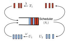
Fig. 2: Timing covert channel in a shared queue.  $T_1$  and  $U_1$  both send packets to a scheduler, and communicate through a covert channel created in the shared queue;  $T_1$  encodes a message on packet arrival times, and  $U_2$  (a partner of  $U_1$ ) decodes this information from queuing delays of her packets.
