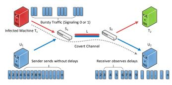
Fig. 1: The insider (Infected Machine  $T_1$ ) encodes the covert messages in the form of bursts. This in turn induces delays into the outsider flow observable by the receiver ( $U_2$ ).
