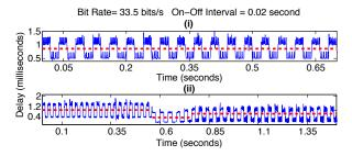
Fig. 4: 1s are represented by an on interval and 0s are represented by an off interval. Alternating 1s and 0s and as were sent. The red line is the threshold line below which we decode a zero and above it is a one.
